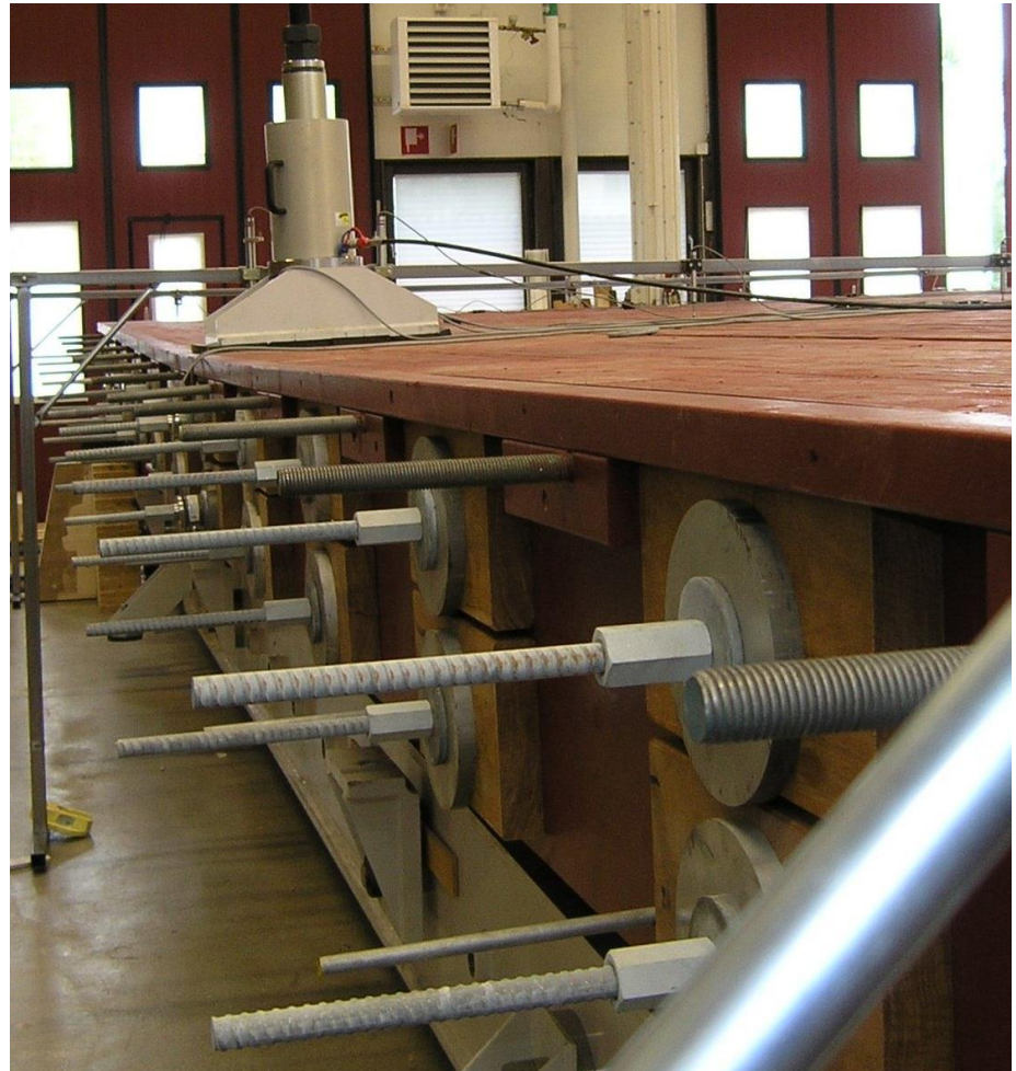
Full scale test, break load over 900kN, photo P-A Fjellström
