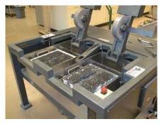
AASHTO T324 - 0/25mm mix - Shear Gyratory Compactor - 20,000 wheel passes - In water at 50°C
